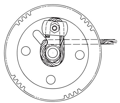
**WARNING:** Keep at least 3 turns of cable on winch drum at all times.
