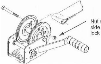
Nut must be on gear side as shown. Use lock nut only.
