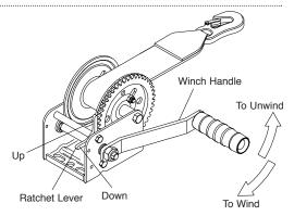
operation to insure the ratchet lever rotates fully without binding.
