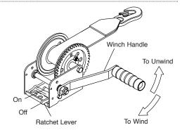
**WINCH MAINTENANCE** — This winch has been fully lubricated at the factory; but, for continued smooth performance and increased life, occasional greasing of gears and reel shaft and an occasional drop of oil on drive shaft bearings are recommended.
