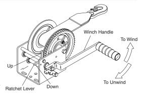
Turn the lever over and reassemble. Do not over tighten bolt. Check operation to insure the ratchet lever rotates fully without binding.
