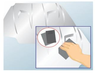
**Sand the finish using a fine-grit sandpaper**. After the primer is set, sand the entire component again with a finer-grit sandpaper such as 180, 220, and 320-grit. After this sanding, continue to apply primer or paint as desired, sanding between each application with a fine-grit sandpaper.
