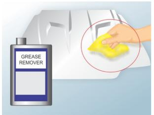
**Clean the entire fiberglass component with a wax and grease remover.** Using this product is especially important when working with a new fiberglass component, as it is necessary to remove the release agent the substance used to pry the component loose from its mold. Wax and grease remover can be purchased from automotive parts stores.
