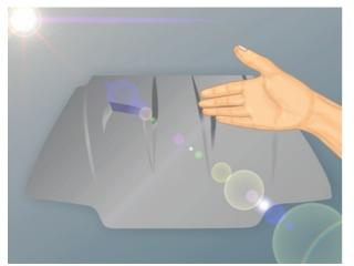
If you are working with a new fiberglass component, it will have a thin layer of gelcoat on its surface. Gelcoat is an epoxy or resin-based compound that is used to line the molds when making fiberglass components.
