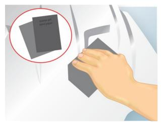
Sand the fiberglass using a coarse-grit sandpaper. For the first sanding pass, use either 120 or 180-grit sandpaper. Mount the sandpaper to a long sanding board for large, flat components. For smaller areas or areas with intricate curves, a rubber sanding block works well to follow the shape of the piece.
