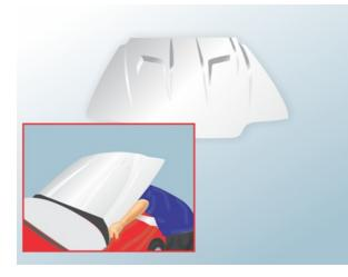
Assemble the fiberglass components, if applicable. If your project consists of multiple fiberglass components (like the body, doors, and hood of a car), assemble them before sanding or finishing. This will allow you to sand continuously between each component, creating a smooth, consistent joint.
