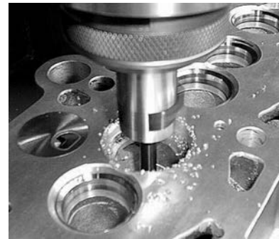
Picture 5 - Cutting the counter bore
