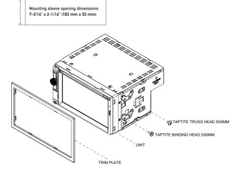
TYPICAL FRONT-LOAD DIN MOUNTING METHOD
