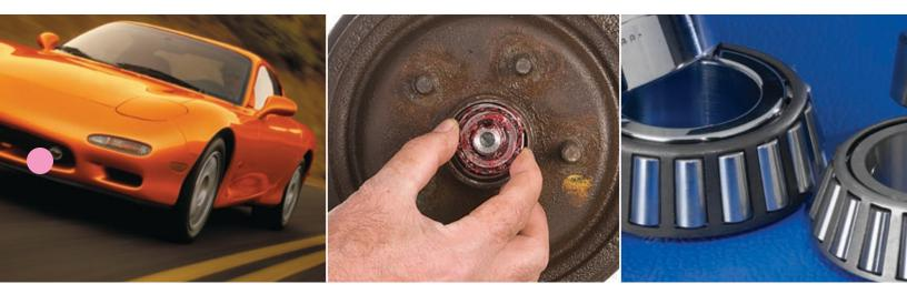
Proper wheel bearing removal and installation is essential in avoiding premature damage to bearings and surrounding components. The following are the steps for replacing tapered single-row wheel bearings in passenger cars and light trucks.
