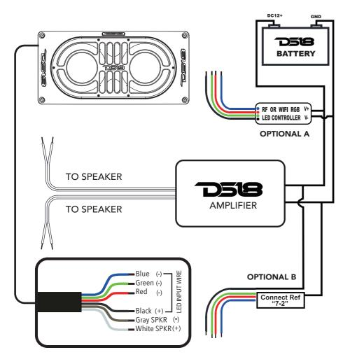
Black Wire "BK" Connected to Battery Positive (+12v) Blue Color Light "B" Connected to Battery Negative (-) Green Color Light "G" Connected to Battery Negative (-) Red Color Light "R" Connected to Battery Negative (-) Purple Color Light "R" and "B" Connected to Battery Negative (-) Yellow Color Light "R" and "G" Connected to Battery Negative (-) Cyan Color Light "R"; "B" and "G" Connected to Battery Negative (-)
