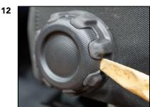
Now we are going to remove the lumbar adjustment knob, using the plastic trim remover tool put in the place shown in the photo and pull it out to release the knob cover.
