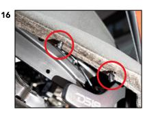
Recline the entire seat back for better access, remove the side of the seat cover by pulling out on the edges, this is secured by plastics retainers.
