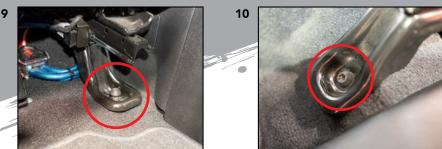
Now locate the 4 screws that hold the seat to the Jeep and remove them using a  $47\,\mathrm{mm}$  Torx tip.
