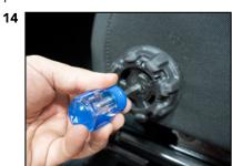
Now we have access to the screw that holds the knob, using the #2 Philips screwdriver remove the screw and take off the knob by pulling it out.
