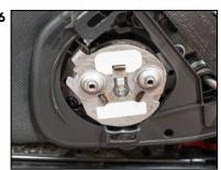
Using the 20mm Torx tip remove these two screws that holds the seat height adjuster handle and take it off.
