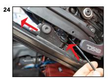
Raise the seat using the lever up to make room between the base and the seat, then pass the mechanism with the wire through in and front as shown in the picture.
