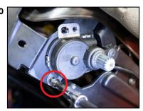
Remove the top and bottom screws that holds the mechanism using the 20mm Torx tip.
