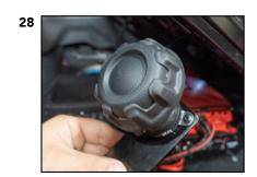
Grab the supplied screws and secure the mechanism with the re-locator bracket, using the #2 Philips screwdriver and the 7mm wrench to tighten those, then put the knob back on the mechanism reversing the process when removed.
