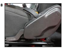
Put the new DS18 handle using the same factory screws and put the cover back, this part would be ready to go.
