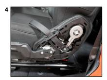
Now just evenly pull the cover out, this is holding on by using pressure clips.
