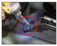
Secure the seat cover back by pressing the pins into their factory holes and put the seat back into position to secure it using the 47mm Torx tip and tightening the all 4 screws back on the seat base.
