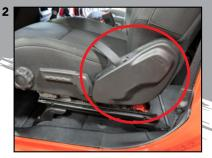
Starts with moving the seat all the way to the front to have free access to this cover.
