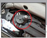
Do not forget to remove in the front corner the seat cover too and then folds up the seat cover to get access to the lumbar adjuster mechanism.
