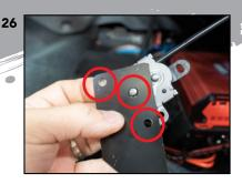
Once its pasted it should be in this position, then take the re-locator bracket and align it as seen in the picture.
