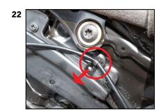
Finish it by removing the last screw that holds the mechanism using this time a 15mm Torx tip, then remove this plastic pin that holds the wire of the mechanism pushing it out.
