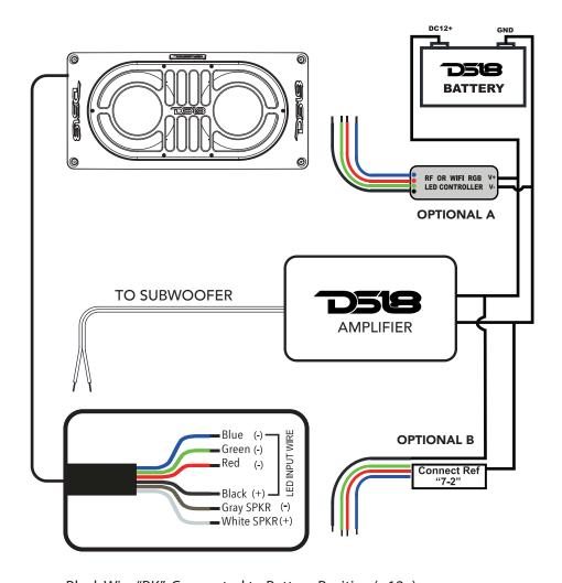
Black Wire "BK" Connected to Battery Positive (+12v)
