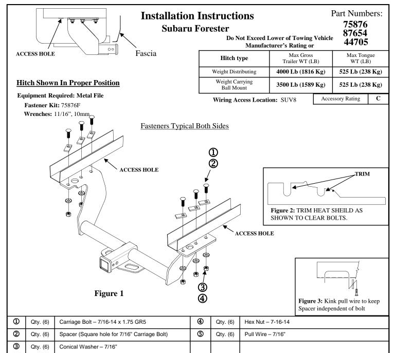
1. Lower exhaust by disconnecting rubber exhaust hanger(s) from hanger bracket(s).
