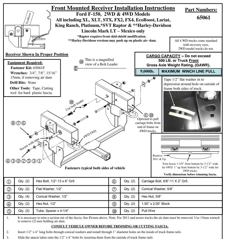
Secure 1/2" flat washers on outside of truck frame rails using tape as shown in the picture above.
