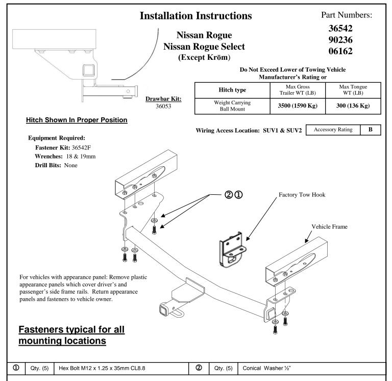
1. Remove and return factory tow hook and fasteners to vehicle owner.
