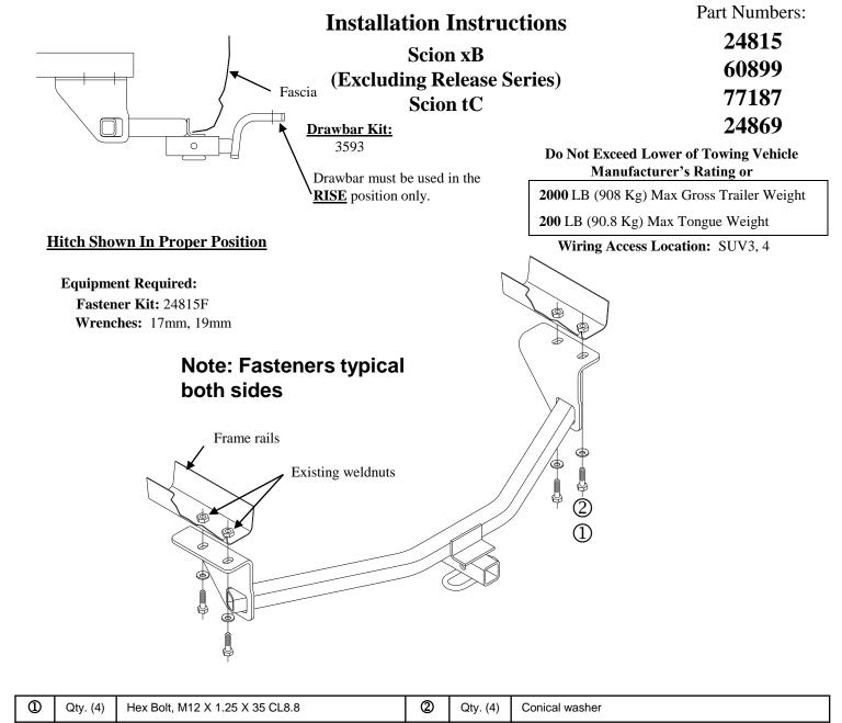
If present, remove the tie down brackets from vehicle frame rail. Return bolts and tie down bracket to owner.
