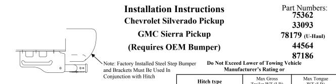
Weight Distributing 8000 (3632 Kg) 800 (363 Kg) **Hitch Shown In Proper Position** Weight Carrying 6000 (2724 Kg) 600 (272 Kg) Ball Mount **Equipment Required:** Wiring Access Location: PU3 Fastener Kit: 75362F Wrenches: 3/4, 7/8, 21 mm Drill Bits: None Factory installed Bumper Bracket - Typical Both Sides Existing Weldnut Typical both sides Frame Existing M14 bolt Note: All Fasteners Typical Both Sides of Vehicle
