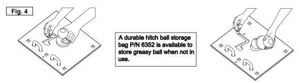
Cover the slot with the magnetic cover provided. This cover will keep road mud and debris out of the bed and away from your cargo.
