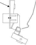
Note: Rotate the hitch for ease of installation.
