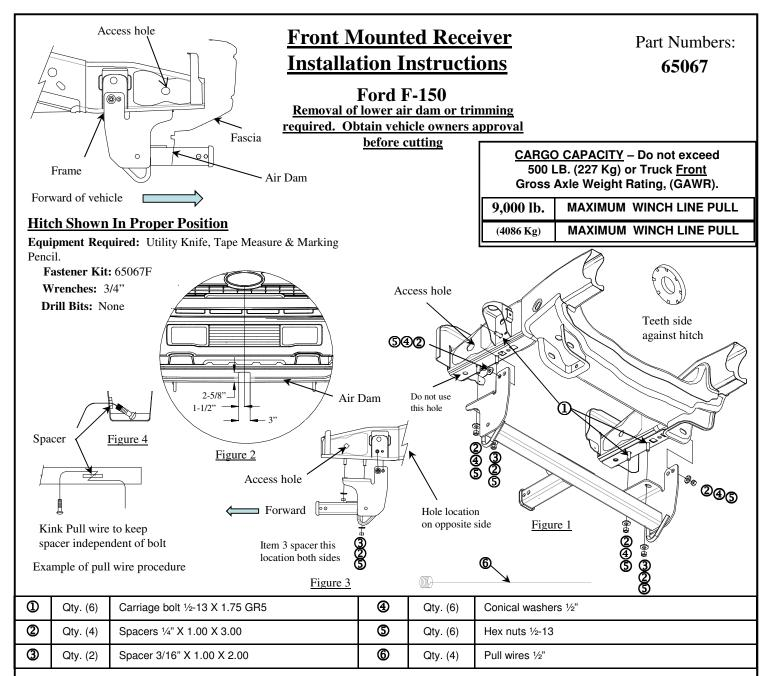
It is necessary to either remove lower air dam or trim plastic air dam to install this hitch. See Picture above. CONSULT VEHICLE OWNER BEFORE REMOVING OR CUTTING PLASTIC AIR DAM.
