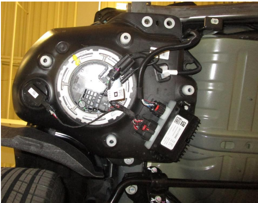
3 bolts, 3 electrical connections
