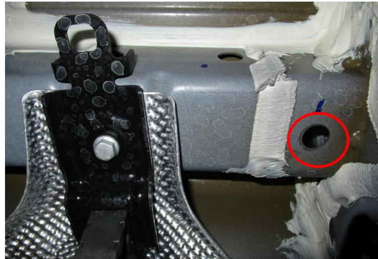
**3. Lower exhaust hanger and caulk removal** – use 13 mm socket to remove (1) bolt from exhaust hanger each side and lower the muffler temporarily, see **Figure 2**. Use a support or bungee cord to keep muffler from getting damaged. Use utility knife to remove caulk near rear mounting holes, see **Figure 3**. Bend down or cut off the legs of exhaust hanger bracket both sides for easier installation, see **Figure 3**.
