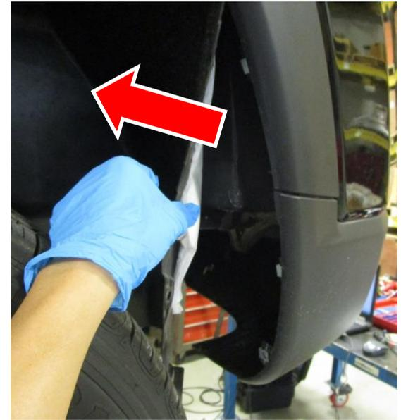
2. Enlarge access hole – peel off (3) plastic covers from holes on the frame rails each side, see [Figure 2](#). Locate the rearmost hole and use die grinder to enlarge the hole size big enough to feed the bolt and spacer each side, see [Figure 2](#). NOTE: for the models with factory tow hook, use 21 mm socket to remove M14 bolts in these locations and save them for reinstallation
