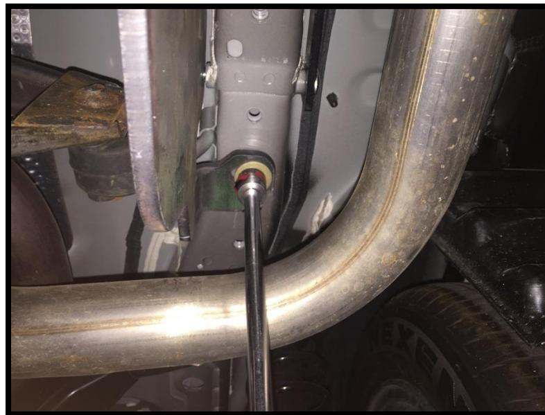
First, tighten the ½-13 GR5 carriage bolts to specifications. Then, tighten the M10 CL8.8 bolts to specifications.
