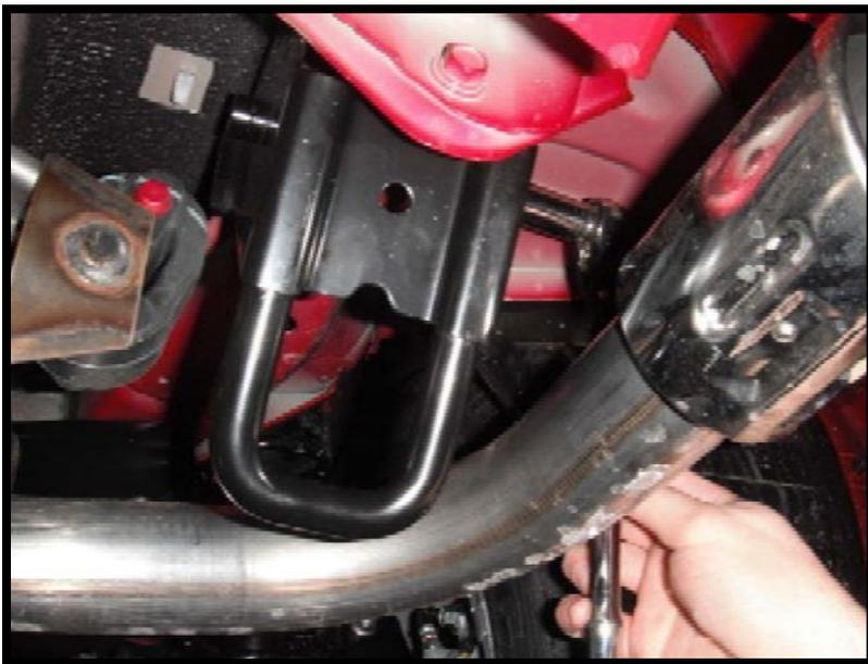
Insert carriage bolts and blocks into existing holes in the side of the frame rails. Adjust carriage bolts to be flush with the inside of frame rails. **Note:** On the driver side, the carriage bolts are installed by reaching between the bumper fascia and over the top of the carbon canister.
