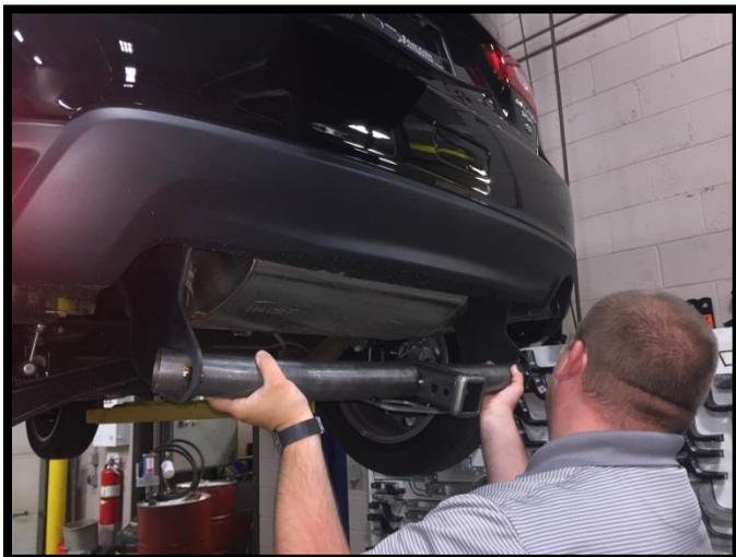
Loosely install the M10 hex bolts with  $\frac{7}{16}$ " conical washers (teeth side toward hitch) into existing weld nuts in the bottom of frame rails.
