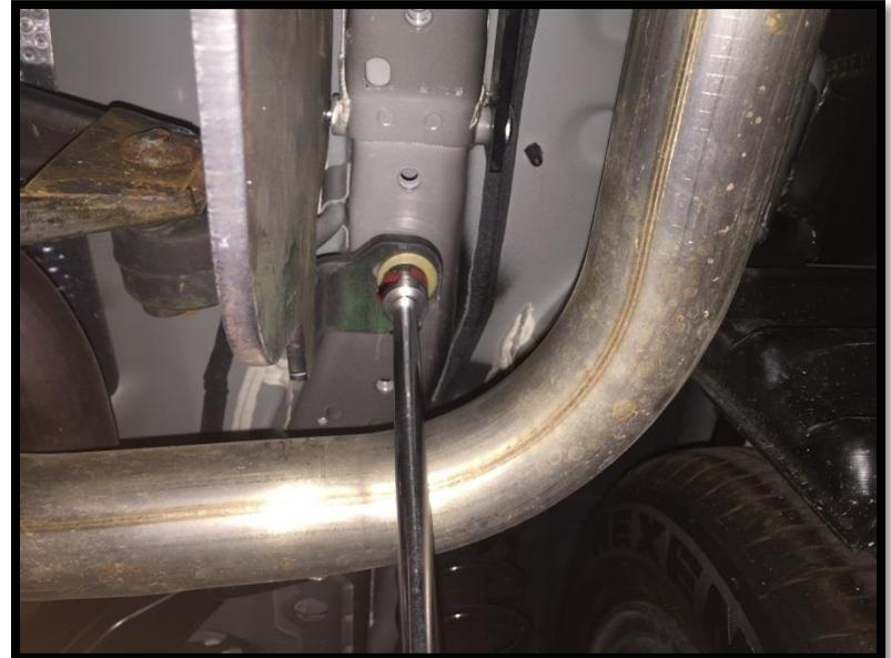
First, tighten the ½-13 GR5 carriage bolts to specifications. Then, tighten the M10 CL8.8 bolts to specifications.
