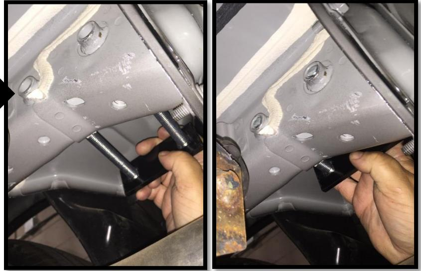
Raise the hitch into position and push the carriage bolts through the holes in the hitch. Loosely install the 1/2" conical washers (teeth side toward hitch) and hex nuts onto carriage bolts. **Tip:** for ease of installation, raise the driver side of hitch first, guiding the flange on side bracket around the carbon canister. Then raise the passenger side into position.
