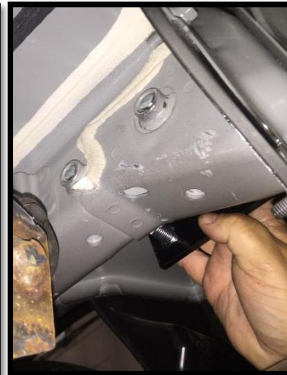
Raise the hitch into position and push the carriage bolts through the holes in the hitch. Loosely install the  $\frac{1}{2}$ " conical washers (teeth side toward hitch) and hex nuts onto carriage bolts. **Tip:** for ease of installation, raise the driver side of hitch first, guiding the flange on side bracket around the carbon canister. Then raise the passenger side into position.
