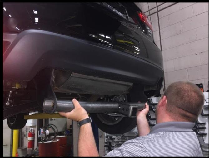
Loosely install the M10 hex bolts with 7/16" conical washers (teeth side toward hitch) into existing weld nuts in the bottom of frame rails.
