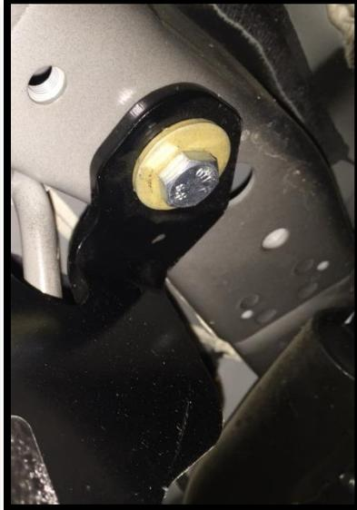
**Tighten all 1/2" GR5 hitch fasteners with torque wrench to 75 Lb.-ft. (102N\*M) and all M10 CL8.8 fasteners to 38 Lb.-Ft. (52 N\*M)**
