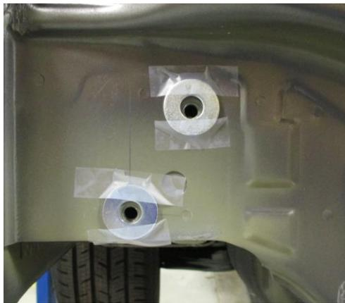
**5. Tighten all M10 fasteners with torque wrench to 59 Lb.-Ft. (80 N\*M) and all M12 fasteners to 76 Lb.-Ft. (103 N\*M).**
