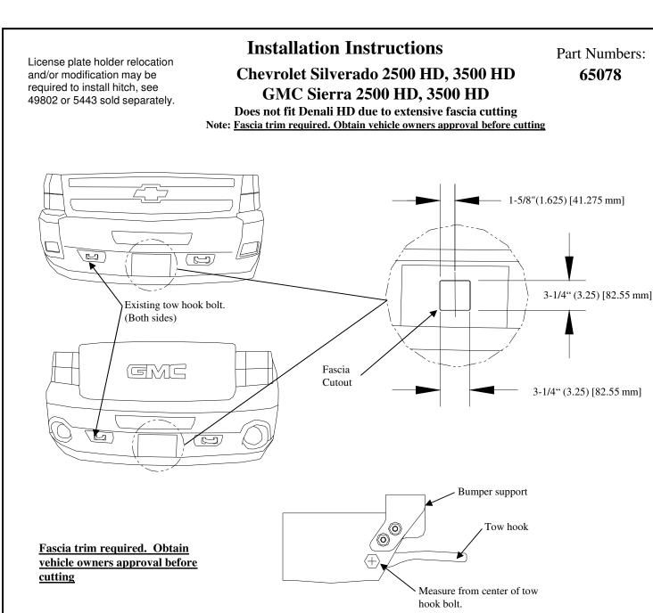
**NOTE:** If front mounted license plate is present, license plate holder relocation, removal and/or modification required to install hitch, see 49802 or 5443 sold separately.
