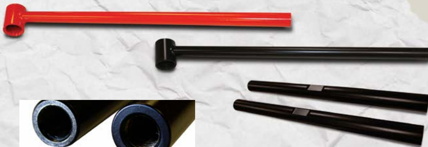
Stock Tie Rod (Hollow Aluminum)
