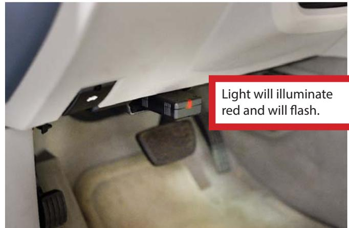
**STEP 6:** The read cycle will occur for 5-10 minutes and when it is complete, the Software Transfer Tool will beep and the LED light will stop blinking and illuminate GREEN.
