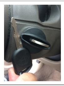
**STEP 4:** Insert the first new transponder key. Turn the key to the ON position but do not start vehicle. Wait for the programmer to beep twice.
