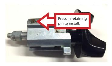
**STEP 2:** Insert the lock into the column. Ensure that the cylinder is fully seated and aligned in the interlocking washer before turning the key to the off position. This will enable the lock retaining pin to extend into cylinder housing.
