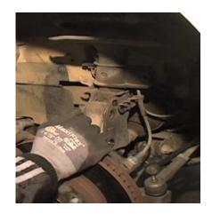
While pulling towards you and pushing on the strut, remove the bottom strut mount from the steering knuckle.
