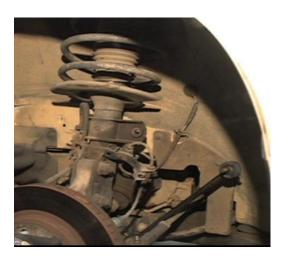
Make sure that the steering knuckle remains supported to prevent damage to drive shaft joints.
