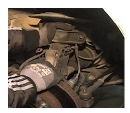
Remove the old strut from the vehicle.
