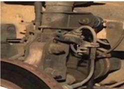
Remove the stabilizer link from strut (if equipped).
