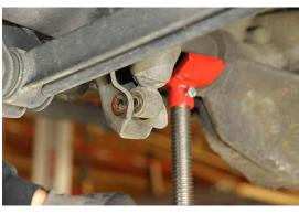
Install lower shock bolt and nut, tighten bolts to factory specs.
