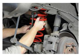
Pull down on the axle and push the coil spring onto the lower spring seat (Small end of spring).
