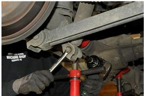
Disconnect the shock from the axle bracket.
