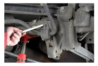
Remove the nut from the bottom of the shock.
