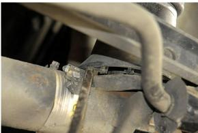
To ensure that the air suspension light does not come on, remove the air spring solenoids from all air springs and reconnect them to the vehicle electrical connectors.
