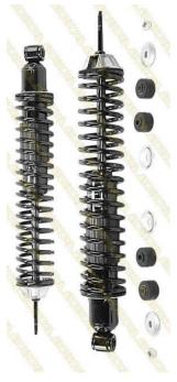
Install the shock into the upper mounting first. Add the other bushing then washer.
