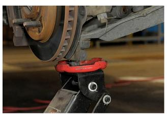
• Disconnect the upper control arm, this will make the removal and installation easier.
