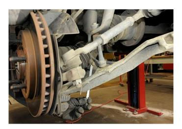
• Remove the lower shock bolt.
