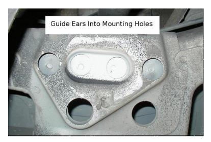
Continue jacking until the spring is compressed enough to reinstall the three lower spring seat mounting bolts. When reinstalling bolts, reverse the bolts so that the nuts are on the
