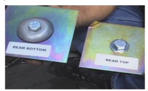
• Install the supplied bottom spring support by putting the bolt and washer through the bottom of the spring seat and install the plate and hardware on top of the spring seat. Tighten nut and bolt.
