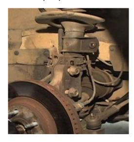
While pulling towards you and pushing on the strut, remove the bottom strut mount from the steering knuckle.
