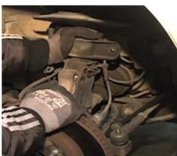
Remove the old strut from the vehicle.
