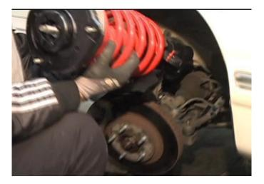
Push the mount studs up through the strut tower. Hand start the nuts onto the studs. Do not fully tighten.
