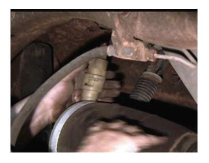
Remove the lower shock mounting nuts and pull the shocks away from the axle. This will allow the axle to lower during the installation of the new springs.
