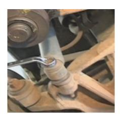
Remove the sway bar end link. This will allow the lower control arm to move downward more and assist in the spring install.
