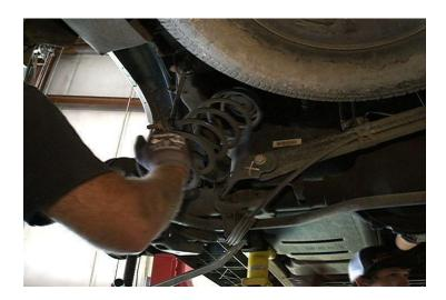
Retain both rubber isolators they will be reused in the installation of the new spring.
