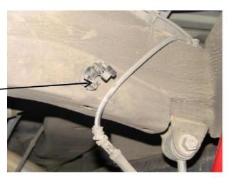
Remove the ride height sensor bracket.
