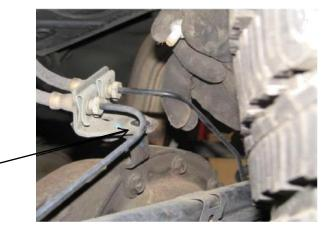
Remove the ABS wire from the frame clip to prevent stretching the wire.
