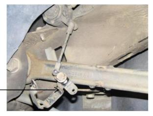
• Remove the ride height sensor bracket.
