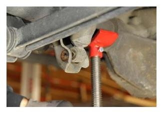
Remove the air spring retaining clip. See figures below
