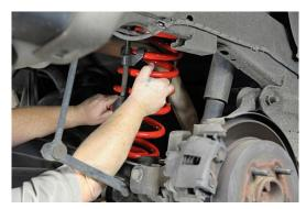
Pull down on the axle and push the coil spring onto the lower spring seat (Small end of spring).
