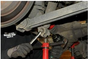
Disconnect the shock from the axle bracket.
