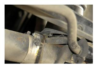
To ensure that the Air Suspension light does not come on, you must remove the air spring solenoids from all air springs and reconnect them to the vehicle electrical connector.
