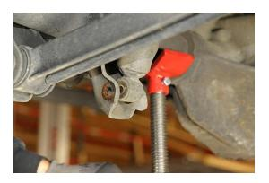
Remove the air spring retaining clip.
