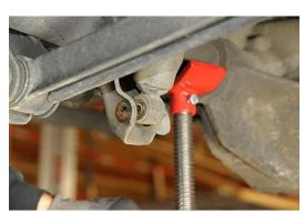
Install lower shock bolt and nut. Tighten bolts to factory specs.
