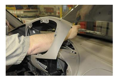
• Lift control module from the instrument panel and locate the dark green wire with the light green stripe. Cut and tape both ends to prevent shorts.
