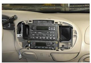
Loosen the main dash cover to access the control module.
