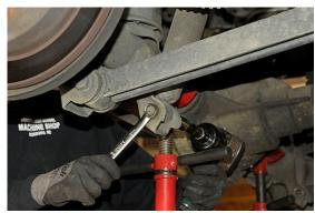
Disconnect the shock from the axle bracket.
