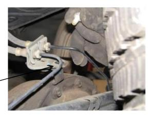
Remove the ABS wire from the frame clip to prevent stretching the wire.
