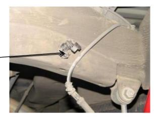
• Remove the ride height sensor bracket.
