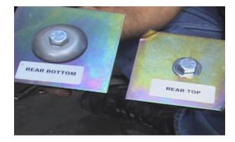
Install the supplied bottom spring support by putting the bolt and washer through the bottom of the spring seat. Install the plate and hardware on top of the spring seat. Tighten nut and bolt.
