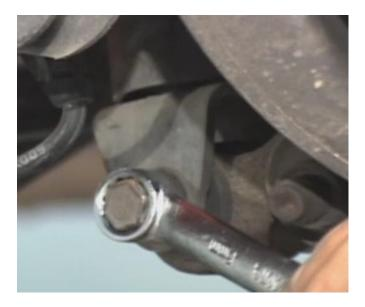
• Remove the top mounting hardware from the old shock.
