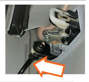
**STEP 7:** Remove the 3 mounting screws retaining the handle to the body using an 8mm socket, and remove the handle from door.
