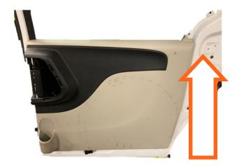
**STEP 5:** Remove access panel on inner panel by gently prying down using plastic trim tool.
