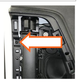
**STEP 3:** Remove inner top corner trim end piece by gently prying in a forward direction using plastic trim tool.
