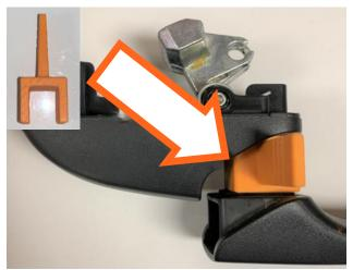
**STEP 2:** With holding tool still in place, reinstall original handle onto door. Have a helper hold handle onto door while installing repair bracket.
