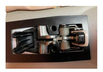
**STEP 4:** Pull on exterior handle in the same direction of handle operation and remove holding tool from handle.
