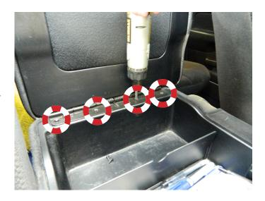
**STEP 3:** Remove the console lid from the center console.
