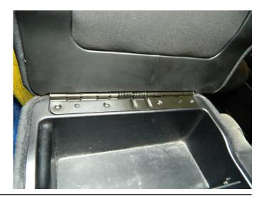
**STEP 2:** Using a Phillips screwdriver or power screwdriver with Phillips attachment, attach the four (4) screws on the bottom of the console lid.
