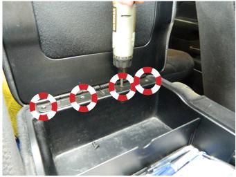
**STEP 3:** Verify that all of the hardware is secure and close the console lid to ensure that it latches properly.
