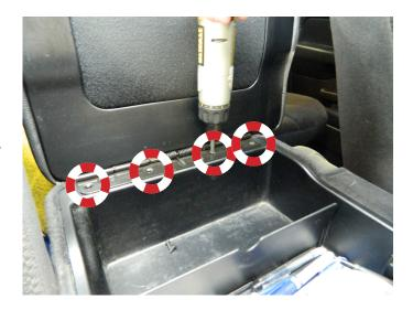
**STEP 3:** Remove the console lid from the center console.
