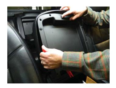
**STEP 5:** Using a Phillips screwdriver or power screwdriver with Phillips attachment, remove the four (4) screws to disconnect the top of the console lid from the center console.
