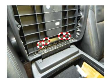
**STEP 2:** Press the underside of the console lid onto the console, making sure to feed the latch through the hole at the top.
