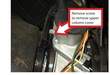
**STEP 4:** Remove upper column cover by removing retaining screw and lifting off of column.
