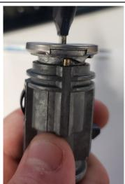
**STEP 4:** Using a small screwdriver, press the brass pin down and rotate the tumbler counter clockwise to unlock tumbler.
