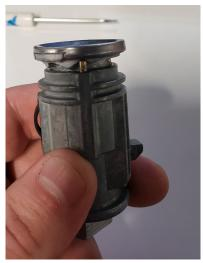
**STEP 3:** Insert supplied key and turn tumbler counter clockwise to the "Accessory" position. **NOTE:** the key will not be removable from the lock cylinder when in this position.
