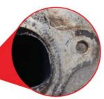
Close up view of broken exhaust manifold bolt
