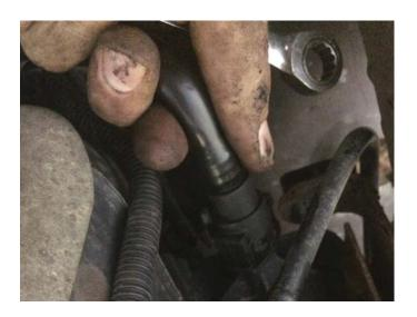
**STEP 3:** Install the two vent valve pipe clips into the existing underbody holes.
