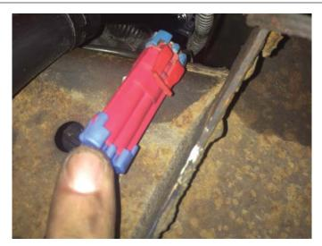
STEP 6: Remove the complete EVAP canister vent valve assembly with bracket attached and discard.
