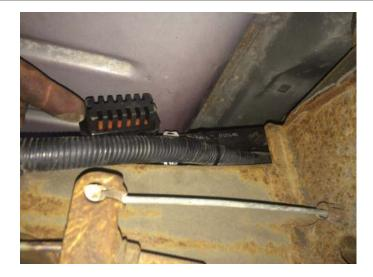
STEP 7: Cut the hose to determined length and install the supplied filter box. Secure using a clamp..
