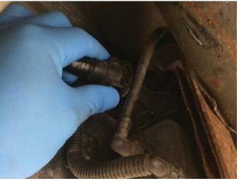
**STEP 4:** Remove and retain the EVAP canister vent valve bracket mounting bolt.
