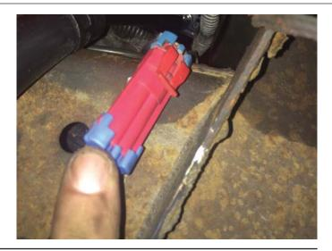
**STEP 5:** Attach bulk 5/8" hose to the vent valve port and secure using a clamp. Run a length as needed along the frame rail routing to the secondary air filter.
