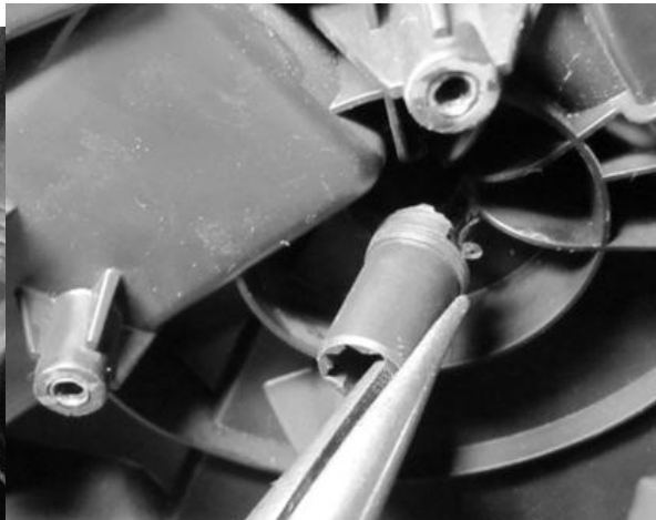
Figure 11- Removing Door Shaft
