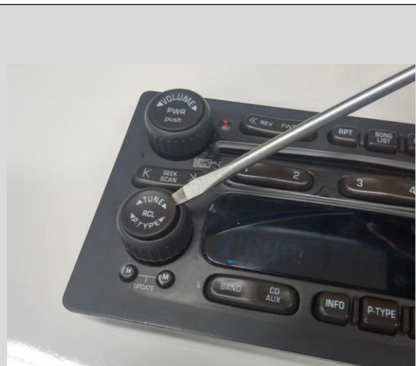
Remove Knob Face First Using Flathead Screwdriver
