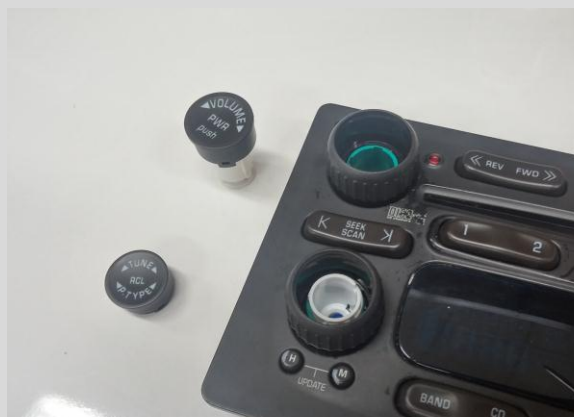
Remove Knob Housing by Pulling Gently.
