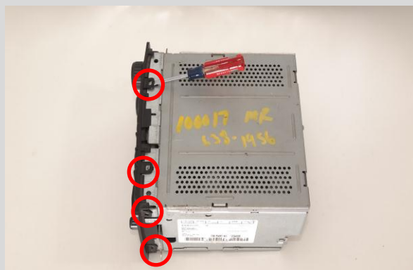
Unlatching the plastic latches using flathead screwdrivers.
